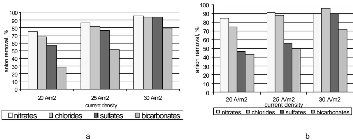
Fig.2. Effect of current density on ion removal from a four-component solution by conventional (a) and monoselective (b) electro dialysis after 2 hours of the process (initial concentration of each component,  $2.5 \text{ eq/m}^3$ ).
