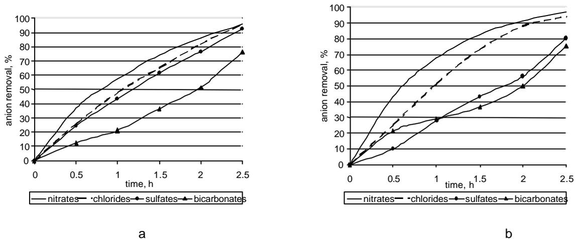
Fig.3. Concentration variations for particular ions in the diluate during conventional (a) and monoselective (b) electro dialysis (initial concentration of each component,  $2.5 \text{ eq/m}^3$ ;  $i = 25 \text{ A/m}^2$ ).
